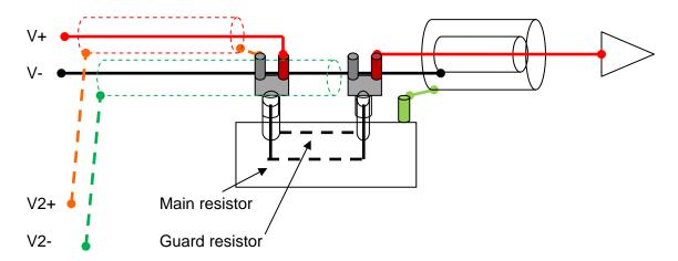
To reduce leakage, connect a second voltage source to the resistor guard high and low as shown in the dotted lines. Generally, the V2- will be at ground potential. Set the V2+ guard voltage to equal the V+ measurement voltage.
